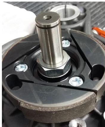
Heat the bell with a blow-dryer on both sides, about 30 seconds per side, using proper heat-resistant gloves
